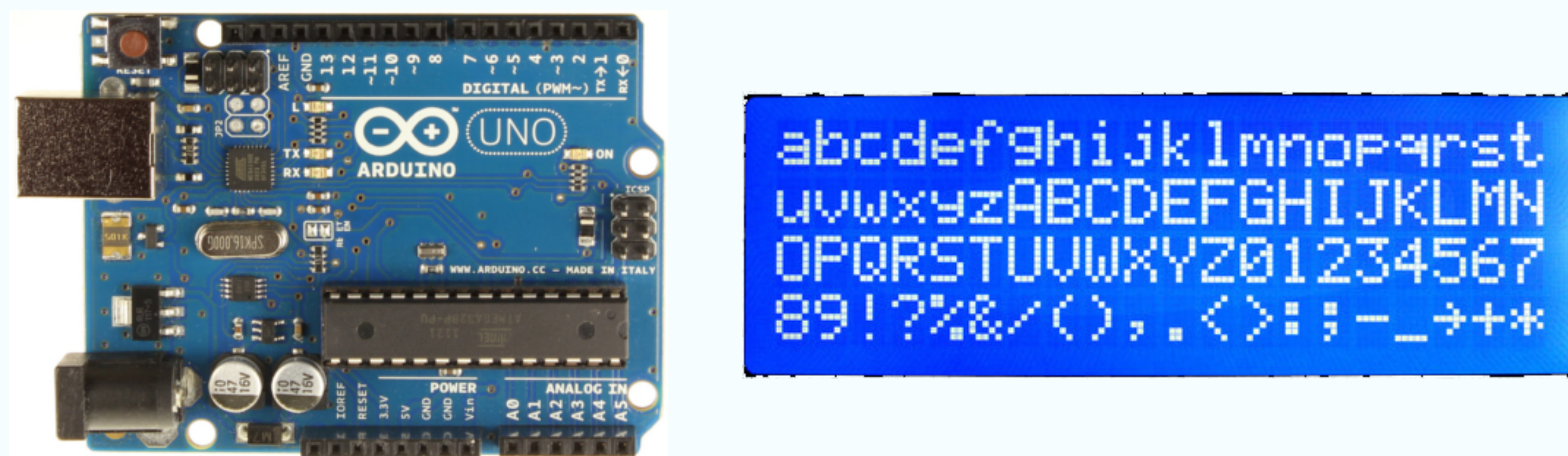
Figure 1. A microcontroller such as an Arduino (left) and an LCD display will be used to display varying messages to building occupants to encourage them to turn off the lights when appropriate.
