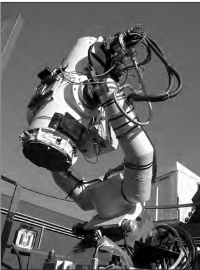
The Télescope à Action Rapide pour les Objets Transitoires (Rapid Action Telescope for Transient Objects; or, TARTO), which CNES uses to monitor the geostationary orbit. © CNES, France. Reprinted with permission from CNES.
